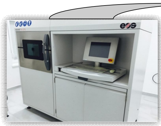
Figure 1. Device for sintering Co-Cr Alloy (EOSint M 280).
